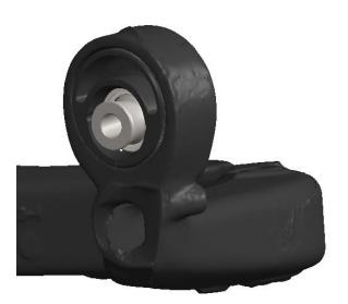
**ii.** With improved anti-squat setting (pick-up points higher on the front mounts) offset the bushing as follows for more clearance in the front mount "bucket" in the chassis:
