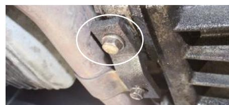
Figure 3: Exhaust retaining bolt (may vary on Diesel Models)
