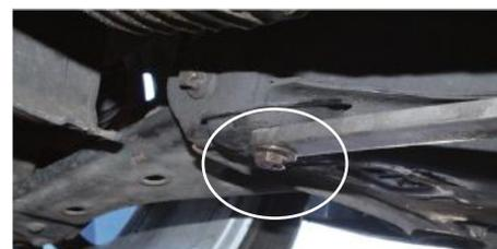
Figure 1: Sub-frame brace bolt (brace may look different on some models)
