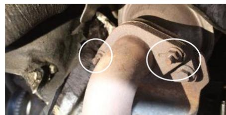
Figure 2: Down-pipe flange bolts (may vary on Diesel Models)
