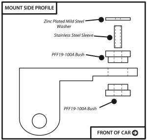
Figure 3- Assembly of 2 front PFF19-100A bushes
