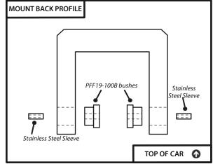
Figure 2- Assembly of 2 back PFF19-100B bushes
