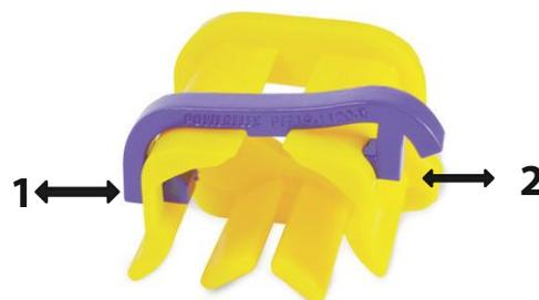
Figure 3 - showing which side to fit first, number 1 and then number 2.
