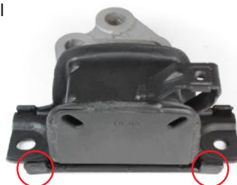
Figure 1: Metal clips to be bent
