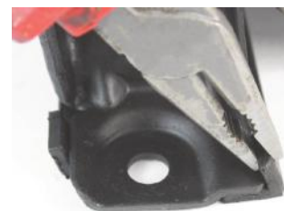
Figure 2: Bend back metal clips
