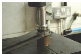
3. Using a press or workshop vice, insert the Outer Shell into the void until it sits flush. Use the Fitting Tool to support the arm as the shell is being inserted.
