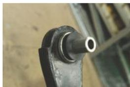
5. Apply some of the supplied grease to the bores of the fitted Polyurethane Bushes and insert the Sleeve into the bore, until it sits flush within the bore.
