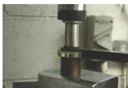
1. using a press or workshop vice, remove the original bush from the arm. the Fitting tool is inserted in the void of the arm to support the arm during this process.
