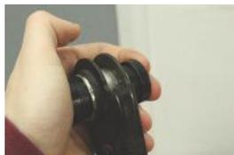
4. Insert a PFR68-131 Bush into each end of the outer shell and push them into the shell until they both sit flush into the bore.
